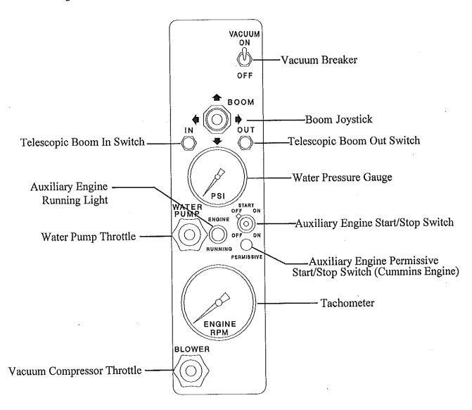
NOTE: The correct way to use these throttles is to screw-in or screw-out knob, not pull and push. However, for emergency shutdown, push center detent button in, and push knob in.
