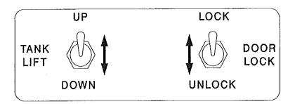
2. To open the rear door, press the door lock toggle switch UP to be sure the hydraulic latches are fully engaged.
